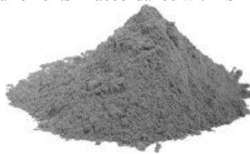
Figure 2.1 Ultra Tech Ordinary Potland Cement 53 Grade
